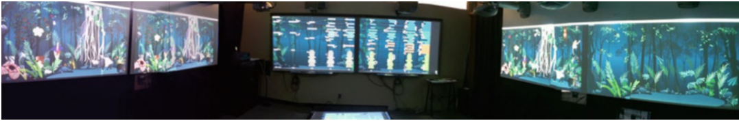
Immersive Environments, Fig. 1 EvoRoom, an immersive simulation for teaching biodiversity and evolution, which consists six projected displays (three on each side) and two interactive whiteboards ( middle )
