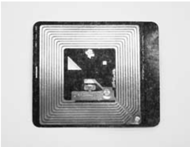
A Radio Frequency ID (RFID) "chip" from 3M. RFID is finding many applications, but has also raised privacy concerns. (3M CORPORATION)
