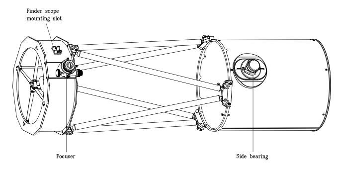
Locate the finder scope bracket and remove the rubber-o-ring on it. Position the o-ring into groove on the finder scope tube.
