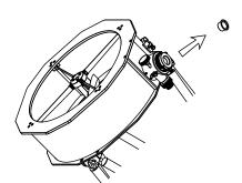
Insert the 1.25" or 2" eyepiece and lightly tighten the thumbscrews to hold the eyepiece in place.
