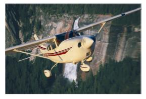
The **Cessna 205**, **206**, and **207**, known primarily as the **Stationair** (and marketed variously as the **Super Skywagon**, **Skywagon** and **Super Skylane**) are a family of single-engined, general aviation aircraft with fixed landing gear, used in commercial air service and also for personal use. The family was originally developed from the popular retractable-gear Cessna 210 and produced by the Cessna Aircraft Company.
