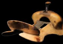
While we honor the tradition of rawhide, Bowden Saddle Tree Company now offers a modern, high-durability alternative: wrapping the fork and the top of the bars with three layers of *eight oz. dual-weave fiber cloth*, then fusing them to a *12 oz. FG mat* located on the bottom of the bars.
