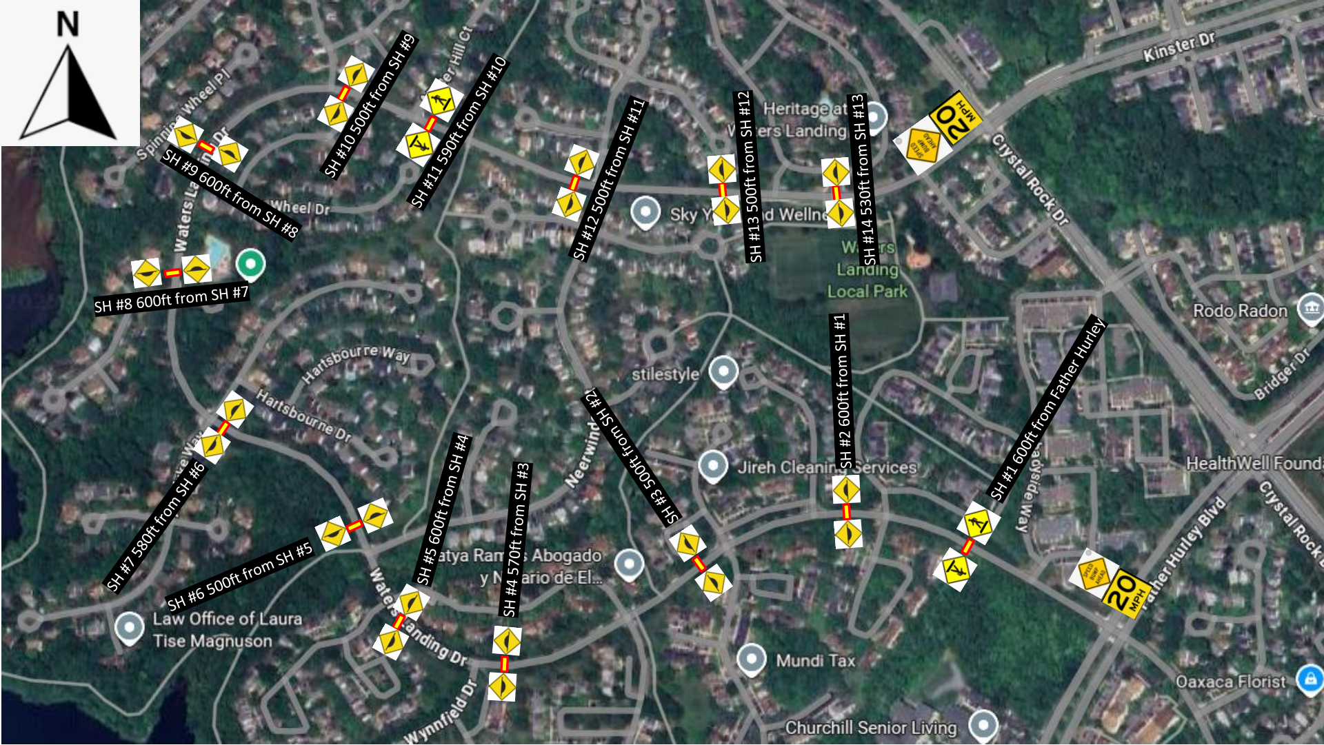
Note: There needs to be min. distance of 500 feet between each speed humps
