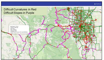
Road-Aware harnesses our proprietary database of highway geometries— a comprehensive collection of road slopes and curves —to provide real-time help tailored specifically for commercial vehicles.
