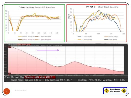
A 3 mile descent averaging -3.8% slope, empty load. Driver B shows lack of speed control downhill with continuous use of service brakes seen in sawtooth braking pattern. Driver A shows a consistent speed pattern resulting in less risky descent.
