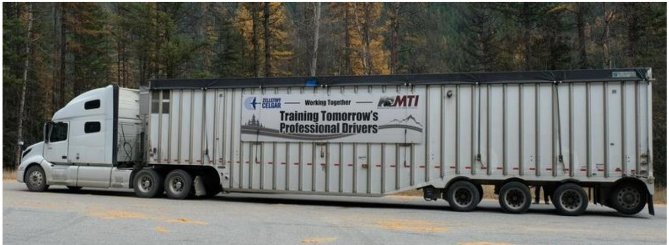
Drivers descended safely in all three runs using only proper gear selection, full use of engine braking and, minor applications of the service brakes, to maintain a +/-1900 rpm for engine safety. In general, the units were able to maintain a 30 mph (50 kph) descent speed in all three runs.
