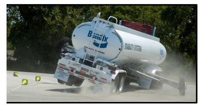
trailer moves through a curve. Livestock loads are among the most unstable loads. Thus, a top driver knows that one of the critical tasks to complete a trip safely is to select speeds in difficult geometries that limit the side forces on the trailer keeping it within the stability envelope.
