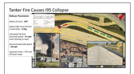
slow the vehicle to limit the side force on the trailer so that it moves through the curve in stable fashion. This example illustrates a case where a driver forgot to slow the rig before the left-hand curve at the bottom of the exit ramp. The tip over threshold speed calculated by *Road-Aware*\* for a loaded tanker is 37 mph for that curve. A safe speed would have been 26 mph.
