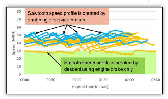
The recommended safe descent speed for this segment of the descent is 30 mph for a truck with a GVW of 80,000 lbs. and engine braking capacity of 350 hp. As can be seen in the charts above most drivers are doing the descent at 40 to 50 mph.
