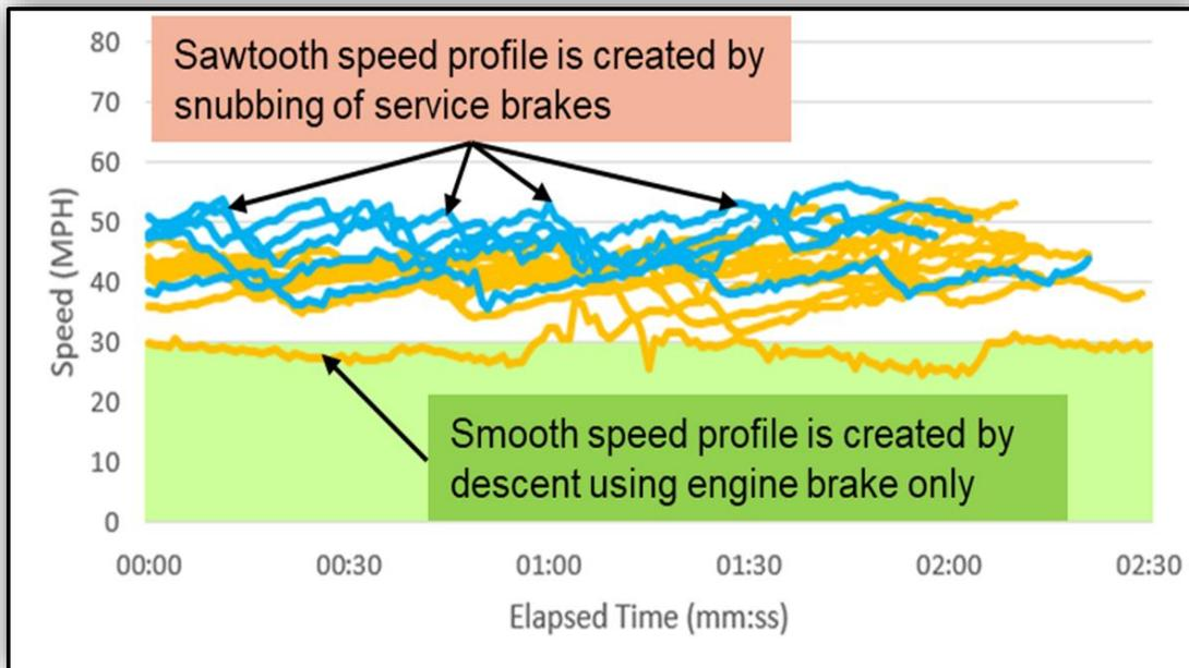
The recommended safe descent speed for this segment of the descent is 30 mph for a truck with a GVW of 80,000 lbs. and engine braking capacity of 350 hp. As can be seen in the charts above most drivers are doing the descent at 40 to 50 mph.
