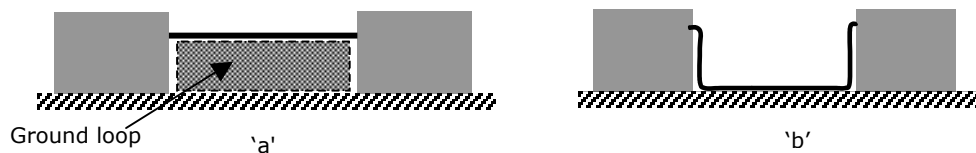
Fig. 11.2 : Reducing CM coupling
