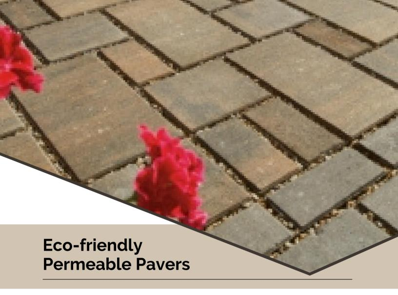
Looking for an eco-friendly solution your hardscape to project? Permeable pavers may be the answer. Permeable pavers allow rainwater to pass around the paver and into the This prevents puddling joints. and flooding, and also filters suspended solids so they don't pollute the water stream.
