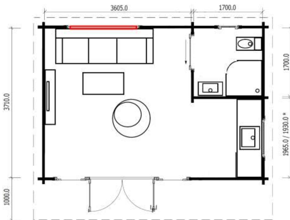
\*dimensions vary based on 45/80mm wall thickness
