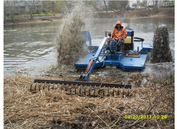
In 2011, FOBP commissioned Lycott to cut and remove all phragmites surrounding Butler's Pond. After cutting the reeds in Winter, hydro-rake machines were deployed in Spring to collect the reeds on the bank for removal by DPW. Annual treatment is required to control re-growth.
