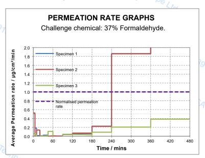
Formaldehyde is determined by discrete sampling; therefore, the permeation rate graph is Technology Europe Ltd not a smooth curve.
