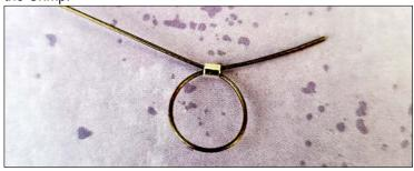
**B.** Pull loop snug around Crimp. Use crimping Pliers to secure Crimp. Trim Tail.
