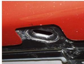
On a C5 Corvette there are 4 cutouts in the fiberglass rocker panels that expose a hole in the frame. There are two on each side. They are meant for a tool called a jacking puck to go into them. You put 1 puck in to each hole so that when the lift touches it, the rocker panels won't be damaged.
