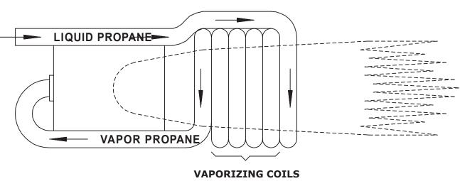
The liquid propane will completely vaporize within 1 - 3 coils, depending on ambient temperature & gas pressure.
