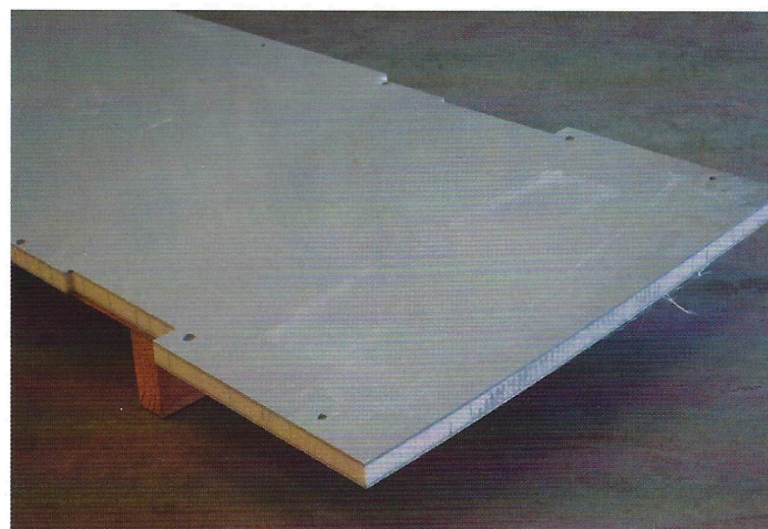
Finished machined deck section.
