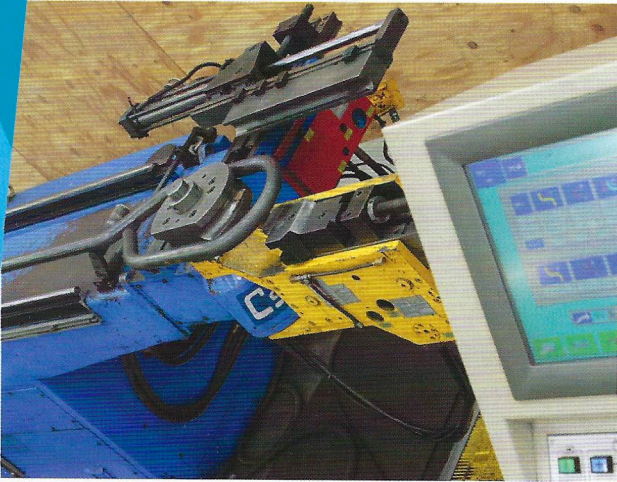
A self loading CNC Tube bending machine is used to accurately bend the teardrop.
