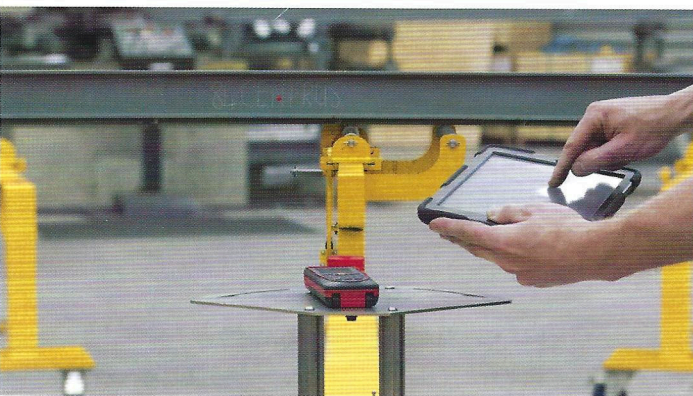
Connected by "Bluetooth" data gathered from laser measuring equipment is transferred to an iPad. Data specific to the "I" beam is then printed and sent with the "I" beam to be used by the installing engineers when assembling the platform on-site.
