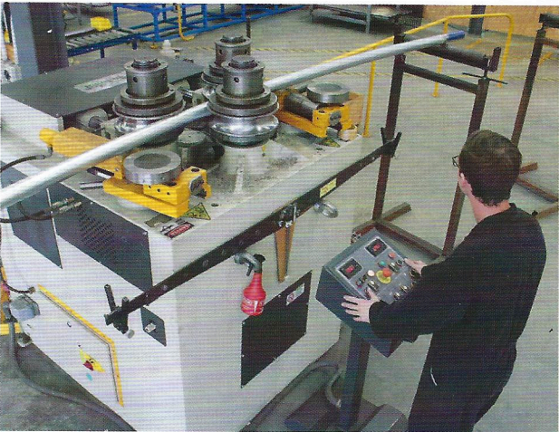
Skilled CNC operators roll galvanised pipe to individual platform specifications.
