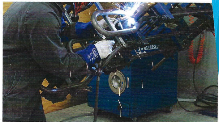
Purpose built rotating jigs present the bail at the ideal angle to get the best possible weld.
