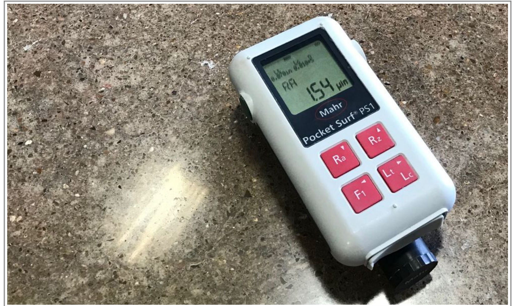
Profilometers measure surface micro texture to provide arithmetic average roughness (Ra) readings.
