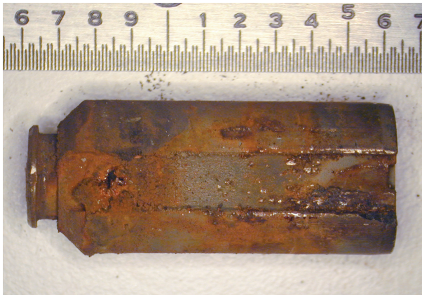
Fig. 14: Solenoid piston in coffee brewer. Corrosion was initiated by acid flux used in copper pipe joining, not the water. Notice severe pitting where chromium oxide coating of stainless steel part has been eroded exposing plain steel allowing corrosion to take place. Defect was detected 6 months after installation. Corrosion of this type will manifest 6 to 18 months after installation.
