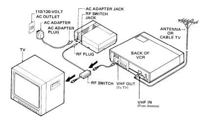
IF THERE IS A CABLE CONNECTED BETWEEN THE VCR AND THE UHF TERMINAL ON BACK OF YOUR TV SET, LEAVE THAT CABLE AS IS.
