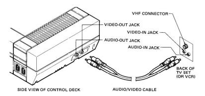
Note! Color coding of TV connections may differ from that of audio/video cable and Control Deck.
