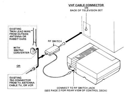
NOTE: If a VCR is already connected between the antenna and the VHF terminals on the back of your TV set, the RF Switch MUST be installed BETWEEN the VCR and the TV as shown below:
