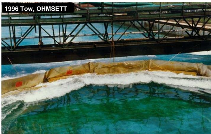
In 1996 Spill-Tain™ fire boom was tow tested at OHMSETT, where it performed very well in oil collecting and retention tests. During these tests it set the facility record for stability and structural integrity by attaining 6 knots, the maximum speed of the facility.
