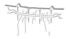
Figure 4. Pin eased area before stitching.
