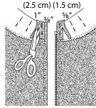
Figure 10. Facing with lapped zipper, before stitching.
