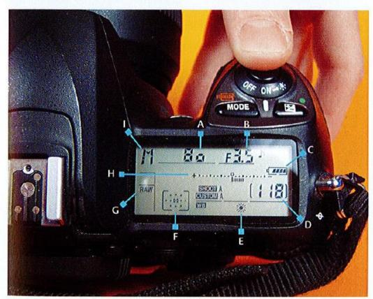
In addition to the large LCD screen on the back, DSLR cameras also have a small LCD screen on the top that is used to display information—not images—to the photographer.
