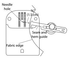
Figure 2. Seam-guide attachment.
