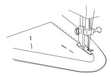
Figure 4. Special seam guide.
