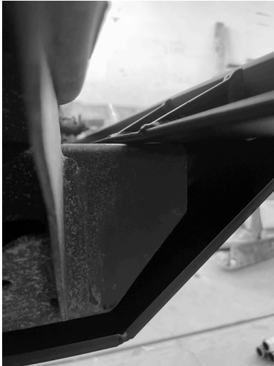
Hang Nguyen Works bumper onto top of stock frame rail. Refer to pic. #16 for another angle.
