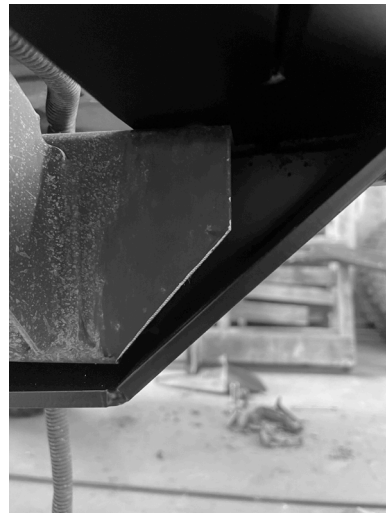
Hang Nguyen Works bumper onto top of stock frame rail.
