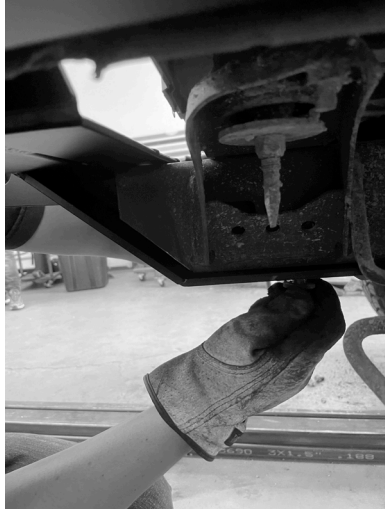
Align Nguyen Works frame mount holes to two stock frame mounting holes on the left and the right side.
