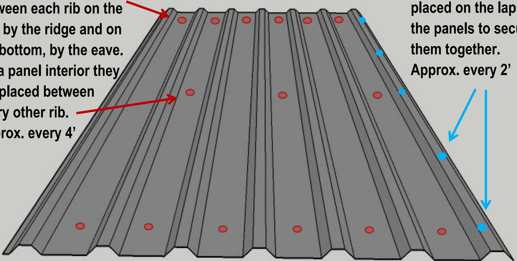
**Fastening:** If you want to pre-drill holes, use a cover sheet to prevent hot shavings to stick to your panels. Drive the fastener so that the washer is compressed securely against the metal. Do not overdrive the fastener as this may cause washer failure which can cause a leak.
