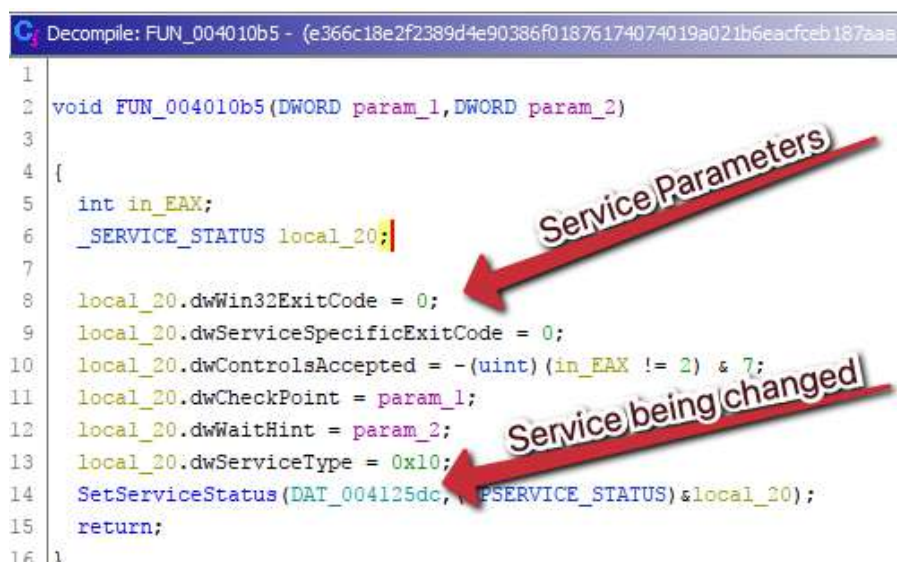
Figure 5.20 – The decompiled view of the API call's cross-referenced function
