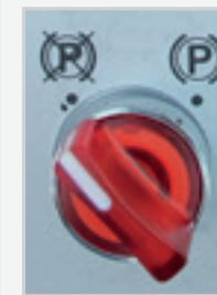
The manual parking brake selector is automatically engaged when the engine is switched off.
