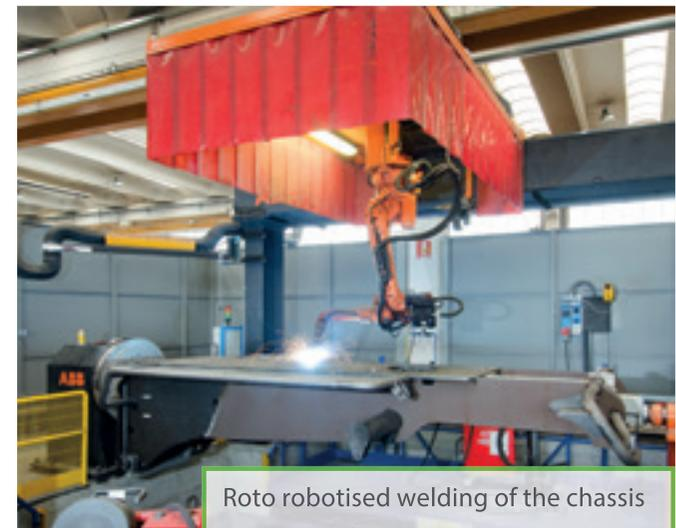
Roto robotised welding of the chassis
