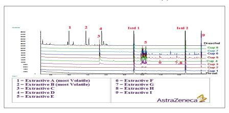
The overlaid chromatograms shown above illustrate that the added leachable have been isolated on the cups of the NGI. And that they are present in droplets that form part of the respirable fraction of the aerosol.
