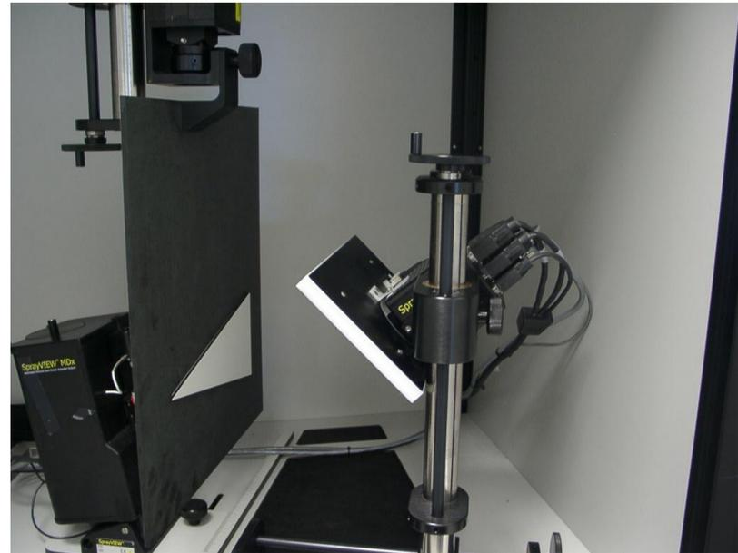
Figure 1: SprayView system set up to measure a plume validation target
