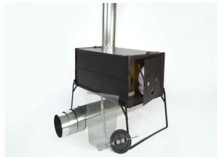
Step 6: Locate stove pipe damper and insert into center piece of stove pipe. Insert the crimped end of the pipe into stove top hole, and stack subsequent pipe accordingly. Hand form the mesh spark arrestor and place it on top of stack.
