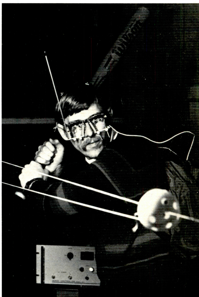
Figure 1. A fastball is simulated when this plastic ball is pulled along the fishing line by the string, which is connected to a motor. The infrared emitters and photodetectors that monitor the eye movements of a subject trying to track this fastball are mounted on the special eyeglasses shown here worn by Dr. Bahill. Two light-emitting diodes used to monitor head movements sit directly on top of the head, and the third is at the end of the stalk.
