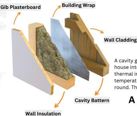
A cavity gap designed to eliminate heat loss and house internal electrical wiring. Our highly efficient thermal insulation prevents extremes of temperature to keep you warm (or cool) all-year-round. They also act as good as sound insulation.
