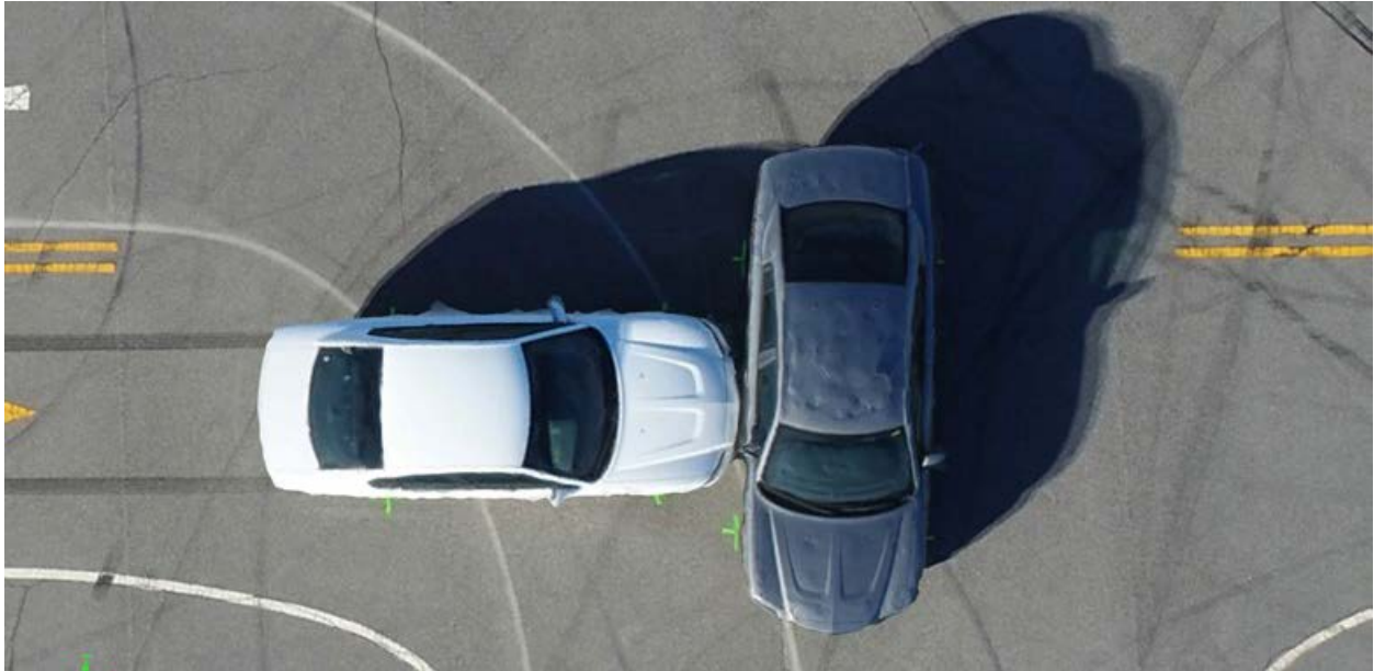
Figure 3-6. Overhead View: Grid + Orbit Trajectory Daytime Reconstruction from DJI Phantom 4 Pro
