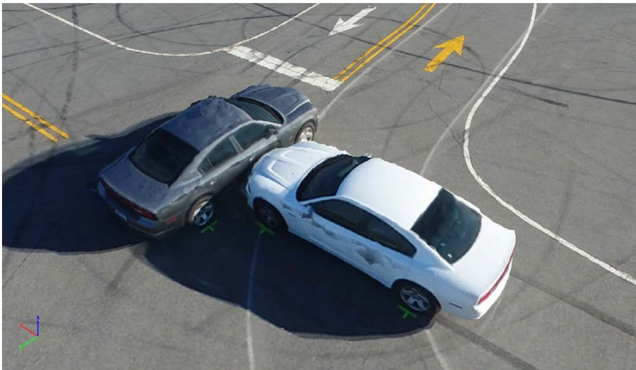
Figure 3-9. Close-Up View: Grid + Orbit Trajectory Daytime Reconstruction from DJI Phantom 4 Pro
