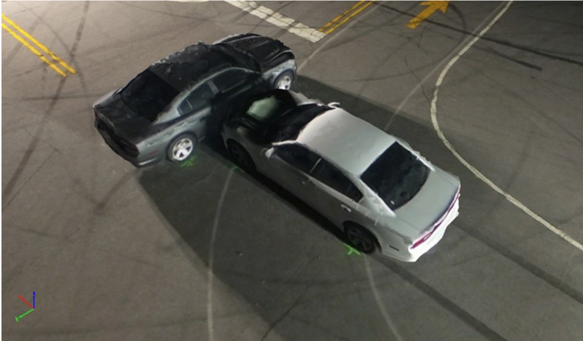
Figure 8-4. Close-Up View: 19:30 Two MLTs Orbit Trajectory DJI Phantom 4 Pro (4-degree sampling) (Day 1)
