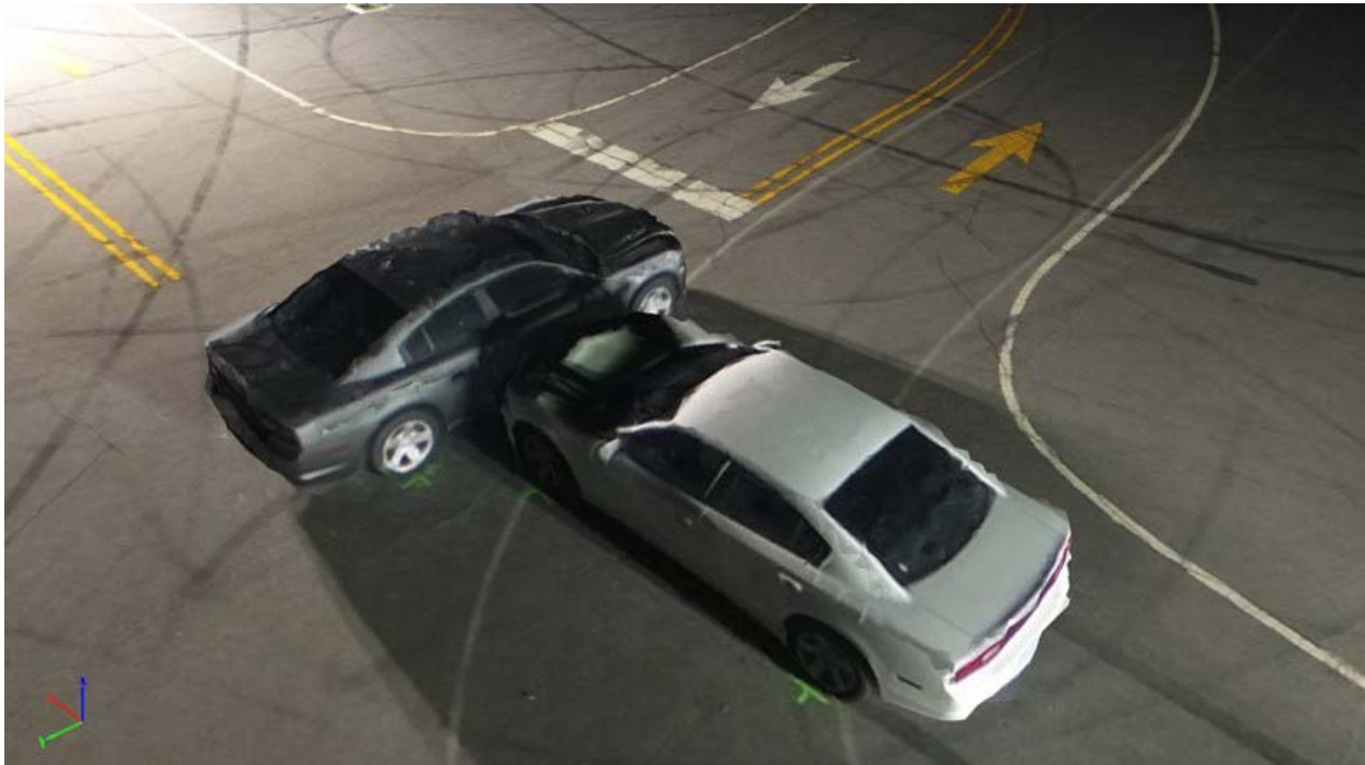
Figure 3-17. Close-Up View: Orbit Trajectory Nighttime Reconstruction from DJI Phantom 4 Pro
