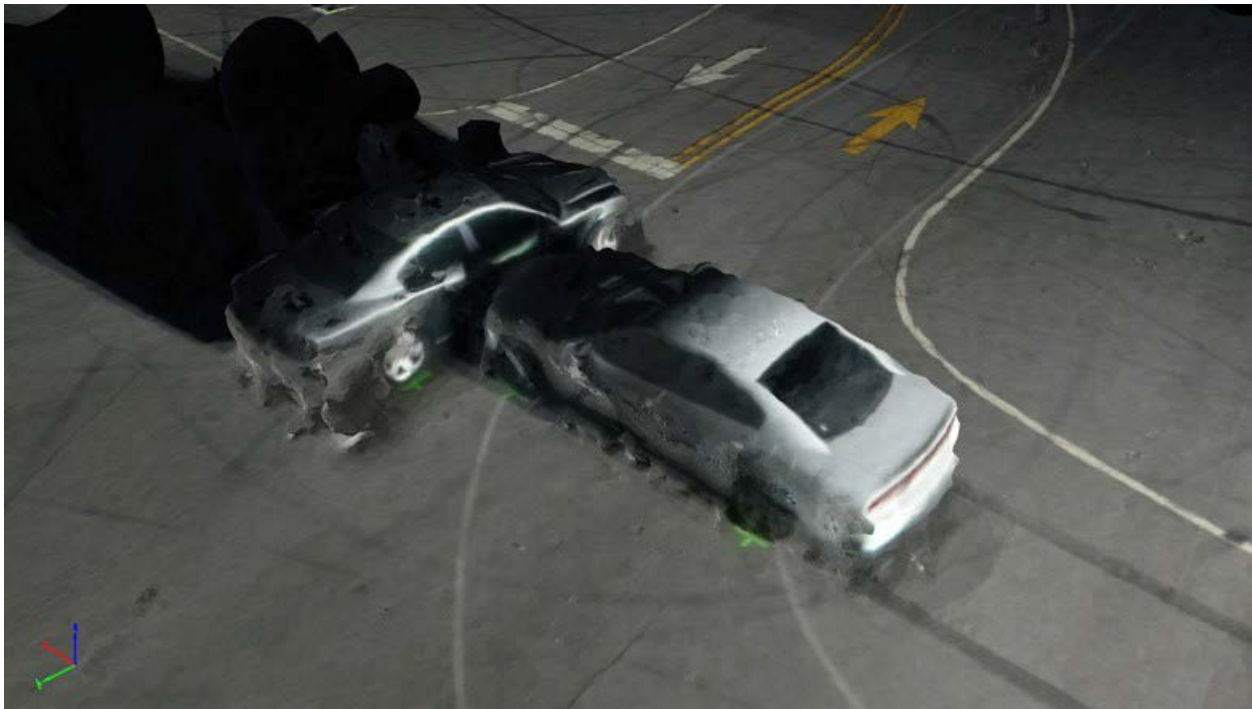
Figure 6-7. Close-Up View: 19:30 One MLT Grid trajectory from DJI Phantom 4 Pro (Day 1). Note the significant scene artefacts in the shadow regions in the upper left part of the reconstruction.
