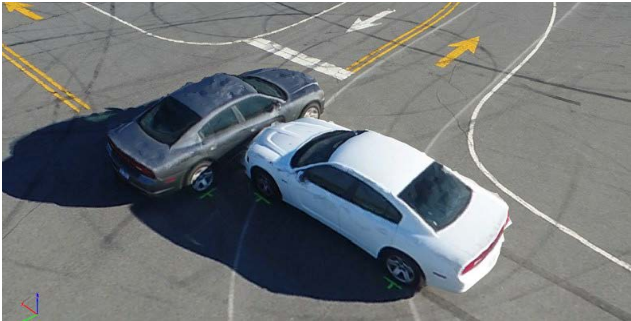
Figure 3-8. Close-Up View: Orbit Trajectory Daytime Reconstruction from DJI Phantom 4 Pro
