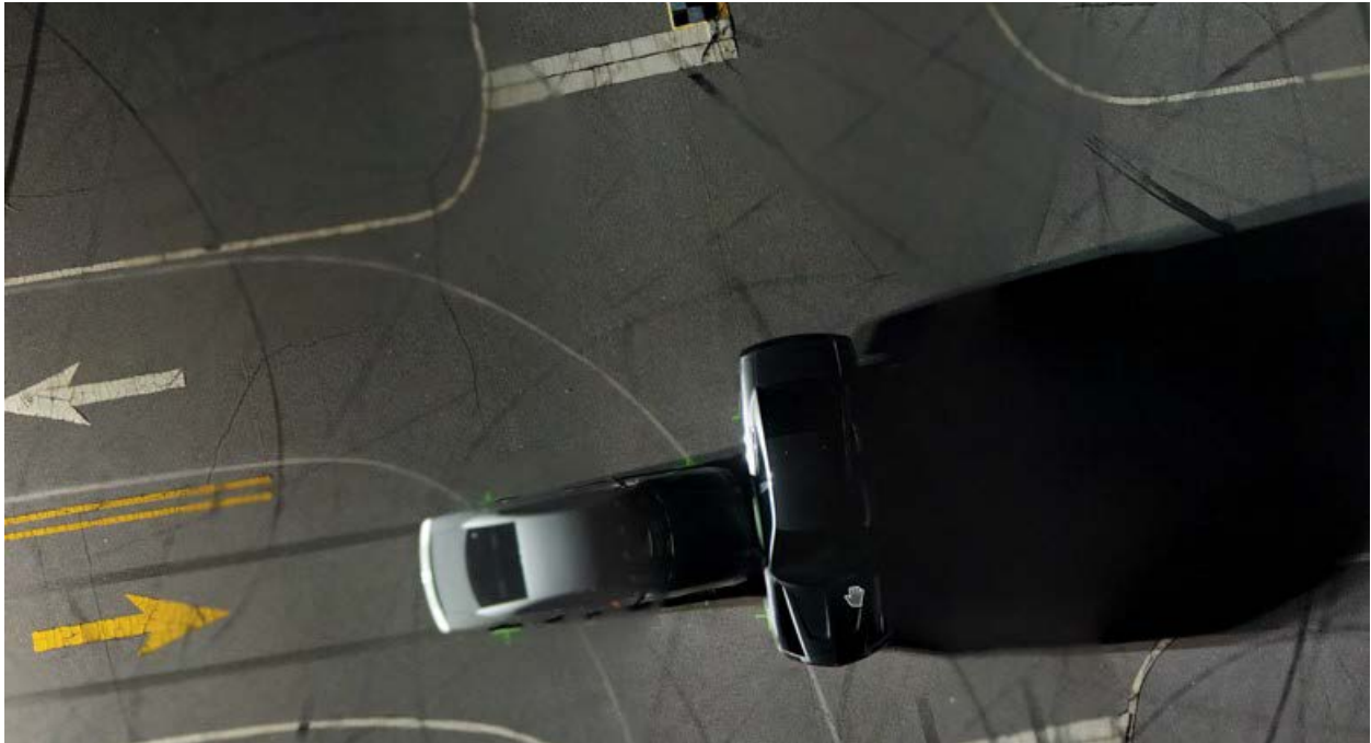
Figure 10-7. Orthomosaic Generated Using Agisoft. Observe the white double line at the top of the image. The left portion is blurry, while the right portion is in focus. Similar variations can be observed in other parts of the image, such as the white double lines at the bottom right of the image.
