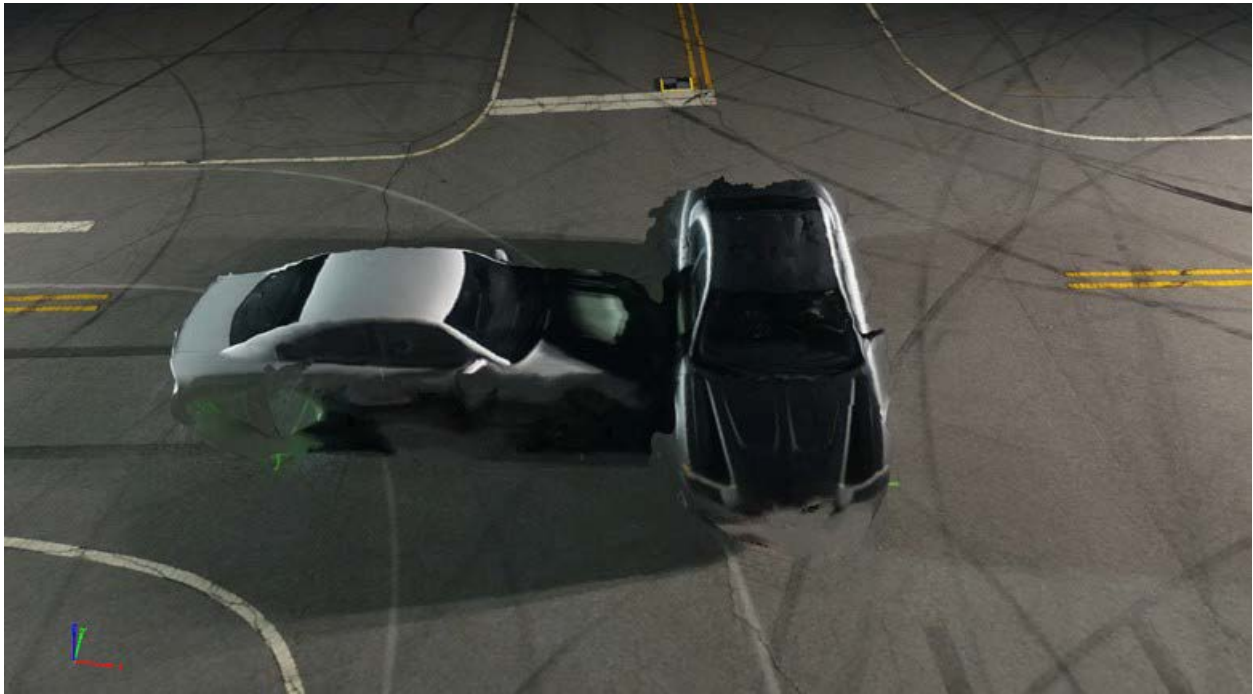
Figure 3-19. Lateral View: Grid Trajectory Nighttime Reconstruction from DJI Phantom 4 Pro
