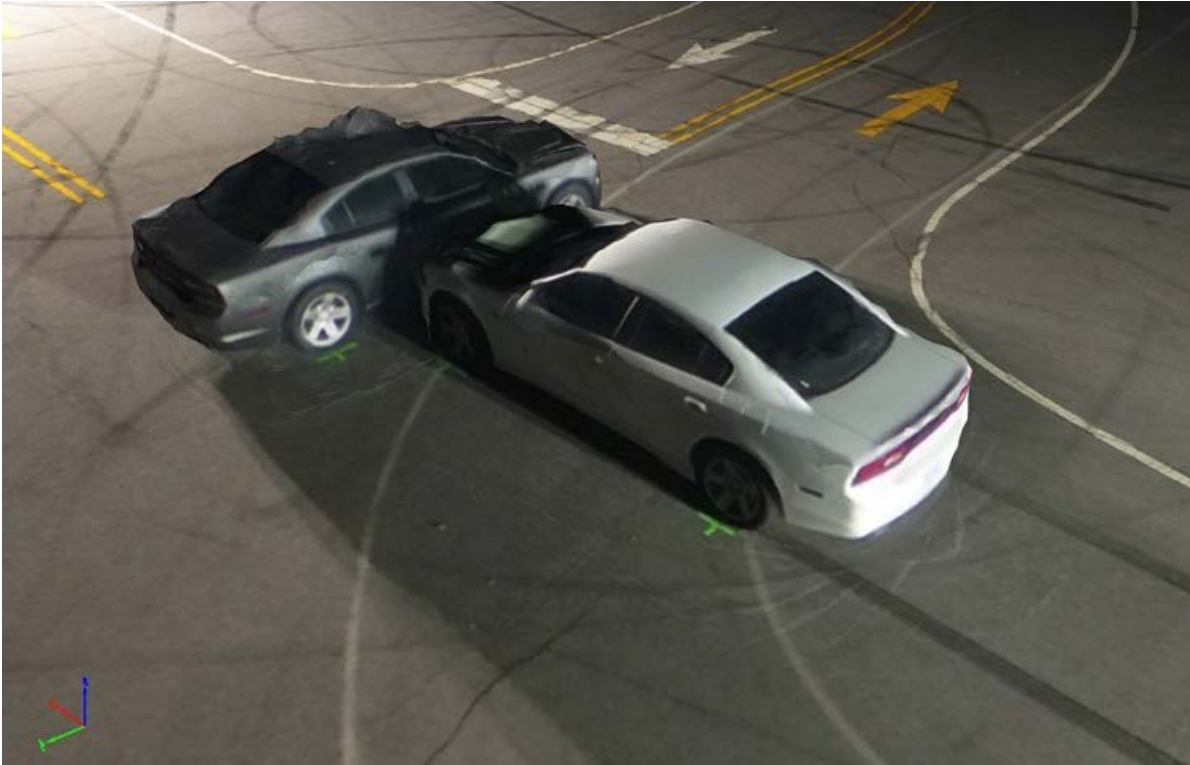
Figure 8-6. Close-Up View: 19:30 Two MLTs Orbit Trajectory from DJI Phantom 4 Pro (16-degree sampling) (Day 1). Note the artefacts on the roof of the gray car.
