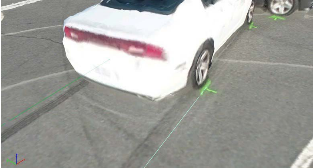
Figure B-1. Start Point of the Measurement for the Rear Right Wheel Skid Mark
