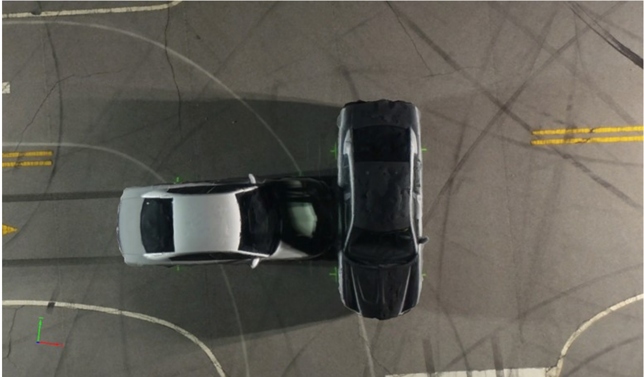
Figure 3-15. Overhead View: Grid + Orbit Trajectory Nighttime Reconstruction from DJI Phantom 4 Pro
