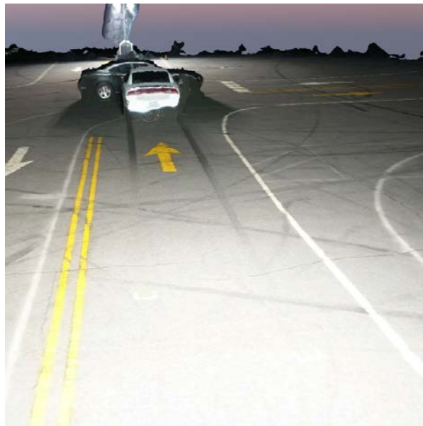
Figure 10-9. Sample 3-D Viewpoint. Note the “waterfall effect” where the rear part of the white car appears to be connected to the road.
