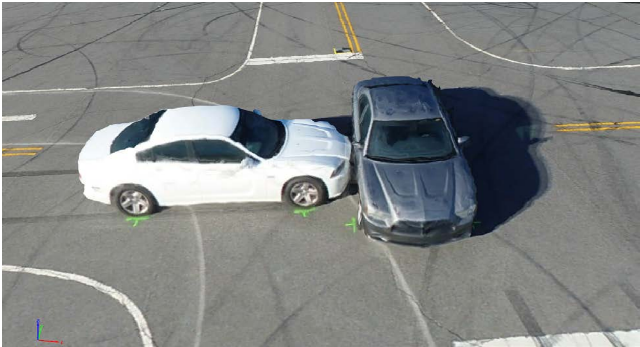
Figure 3-12. Lateral View: Grid + Orbit Trajectory Daytime Reconstruction from DJI Phantom 4 Pro
