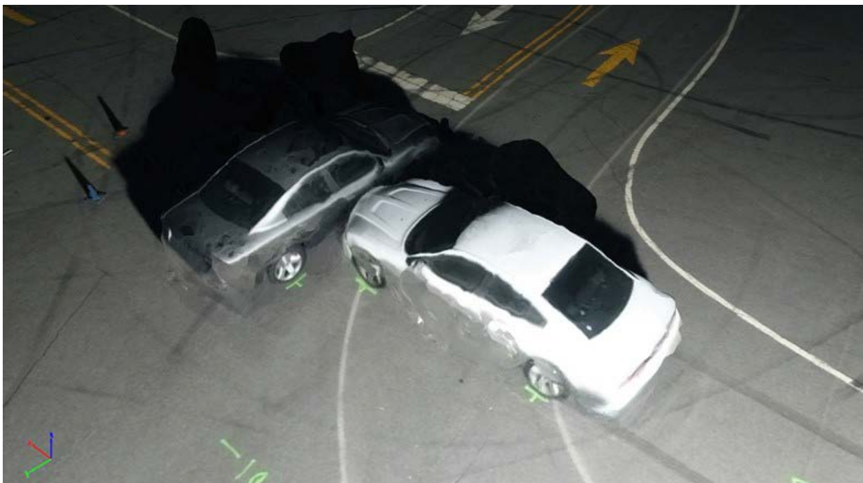
Figure 6-8. Close-Up View: 19:30 ILT Grid Trajectory from DJI Phantom 4 Pro (Day 2). Note the significant scene artefacts in the shadow regions of the reconstruction.
