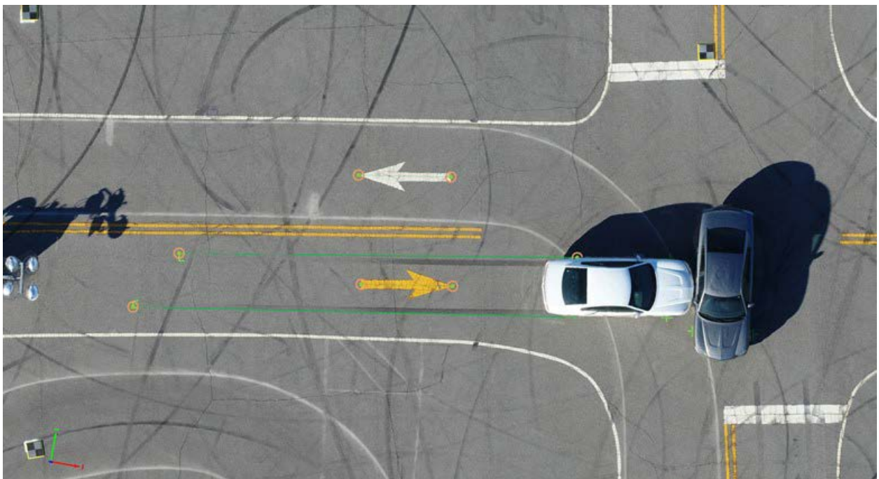
Figure B-4. Overhead View Illustrating Skid Mark Length Measurement
