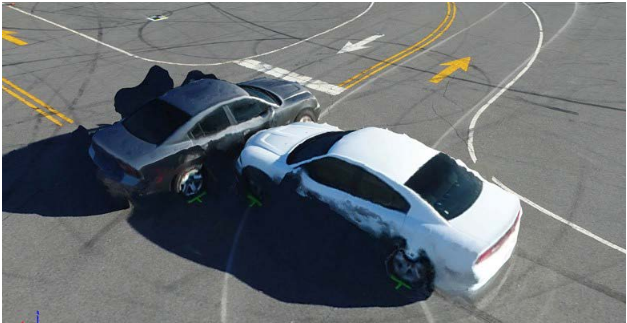
Figure 3-7. Close-Up View: Grid Trajectory Daytime Reconstruction from DJI Phantom 4 Pro. Note the black scene artefacts on the far side of the gray car caused by the shadows.
