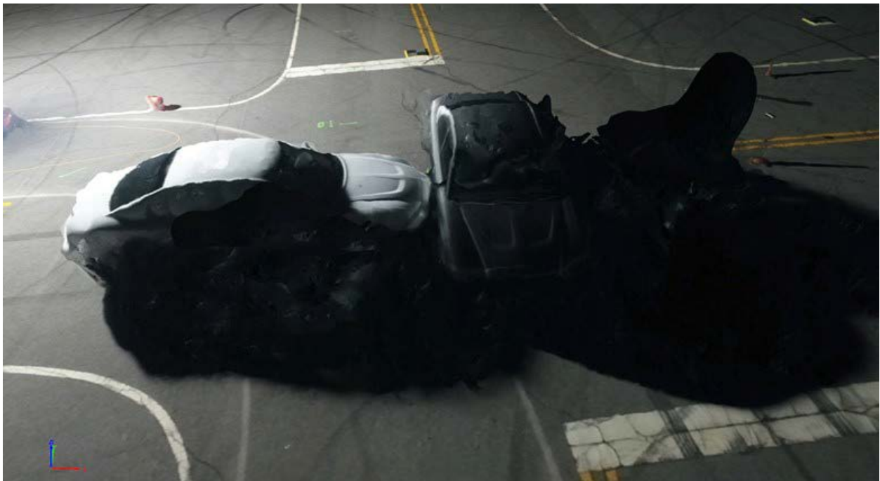
Figure 6-12. Lateral View: 19:30 ILT Grid Trajectory from DJI Phantom 4 Pro (Day 2). Note the significant artefacts in the shadow regions on the right side of the reconstruction.
