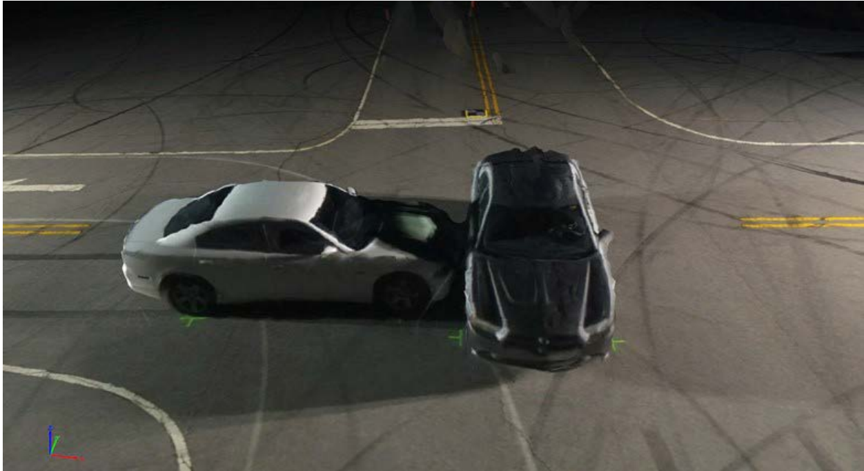
Figure 3-21. Lateral View: Grid + Orbit Trajectory Nighttime Reconstruction from DJI Phantom 4 Pro
