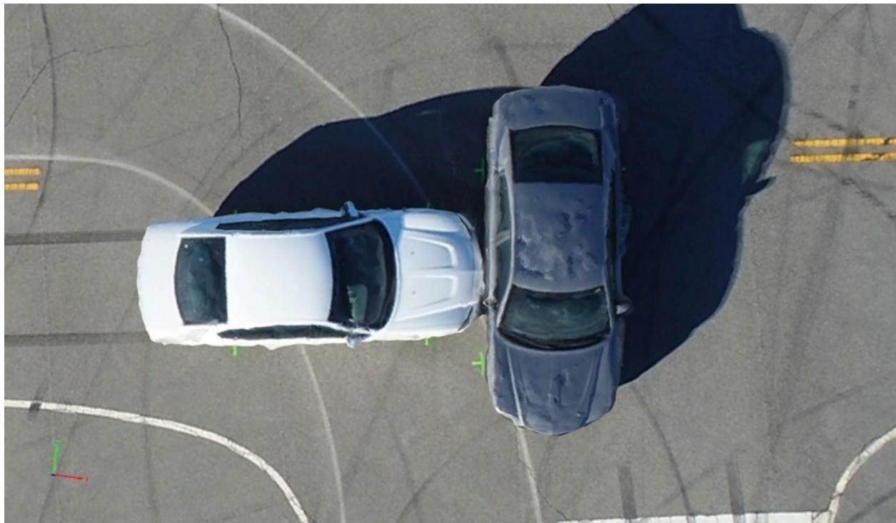
Figure 3-5. Overhead View: Orbit Trajectory Daytime Reconstruction from DJI Phantom 4 Pro
