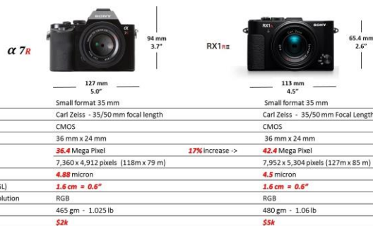
Figure 2: Camera Configuration and Specifications
