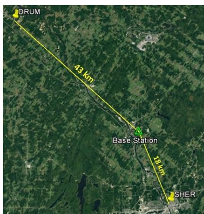
Figure 4: Base Station Location Relative to Cansel Permanent Tracking GNSS Stations
