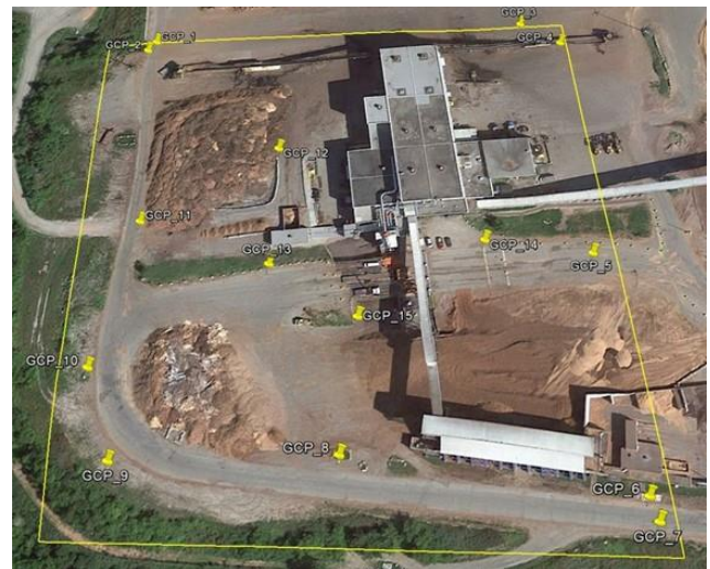
Figure 5: Ground Control Point Layout
