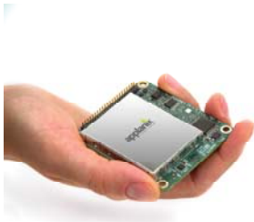
Figure 1: Applanix APX-15 UAV Single Board GNSS-Aided Inertial solution for Direct Georeferencing on UAVs
