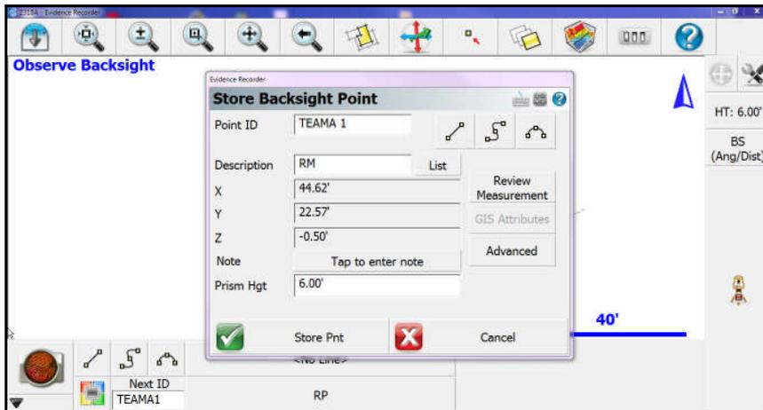
The point ID should be Team A 1. If it does not have this value by default, enter it in the Point ID box above. Make sure the Description is correct and then press “store point”.
