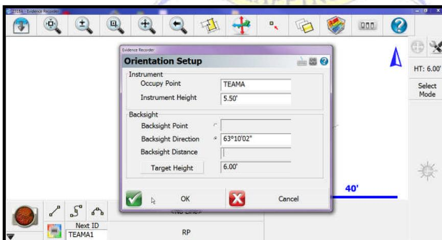
Enter the backsight direction of the reference measurement and the Instrument Height that you have measured and Press “Continue”. Press “Continue” at the next informational screen to see the following.
