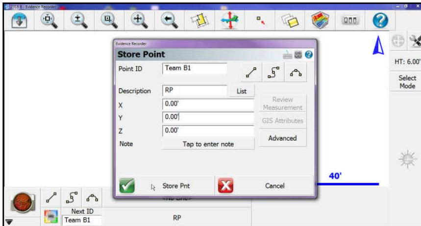
Enter the Point ID, Description, X, Y, and Elevation information for Team A's total station point as provided by Team A and press Store Point as shown in the above example and then press continue at the next screen.
