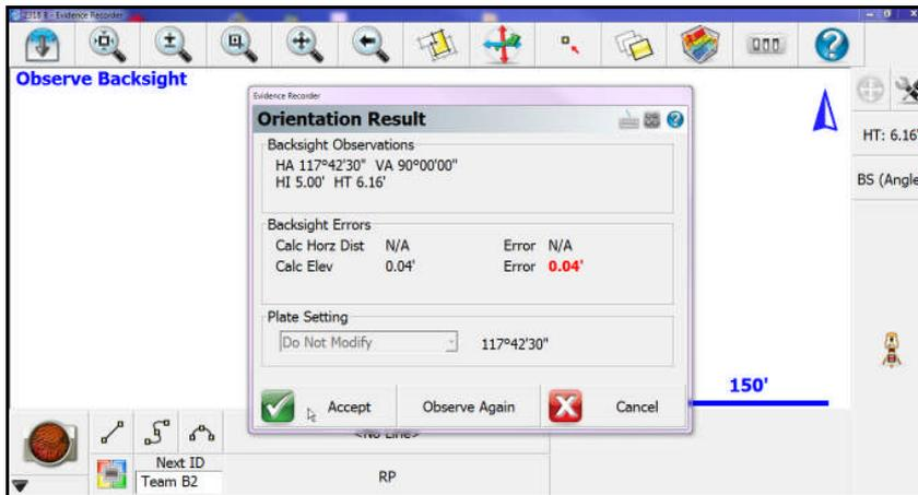
Press the Set Dir Button, Make sure HI and HT are correct and Press Accept.
