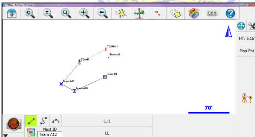
Begin mapping as normal. You can see the alpha-numeric codes for the line above by selecting view point ID’s.
