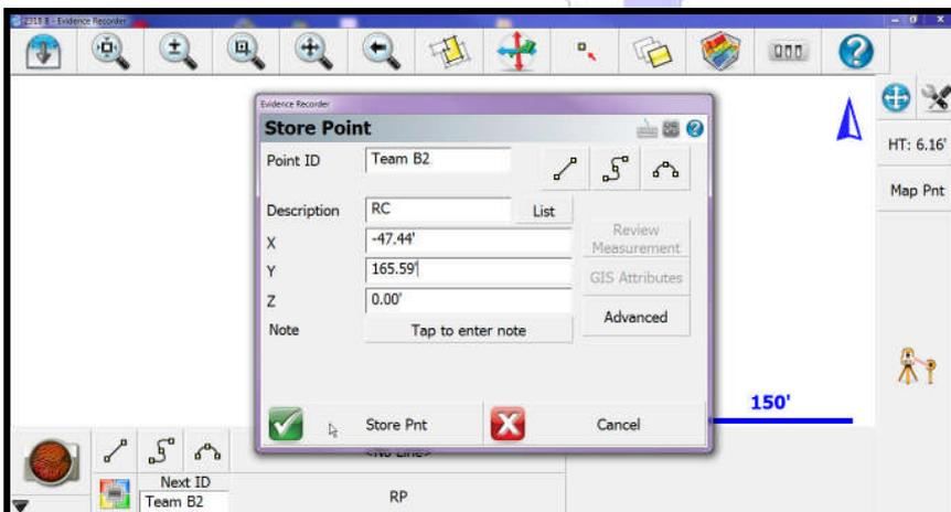
Enter the data provided by Team A for this point which is the Reference Control Point (RC) and Press Store Point when finished.
