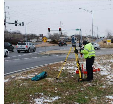
**Figure 7. Photo. Robotic Total Station**
