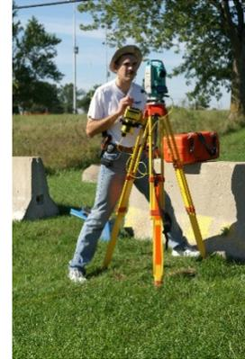
**Figure 5. Photo. Reflectorless Total Station**
