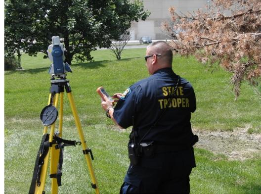
**Figure 6. Photo. Semi-Robotic Total Station**
