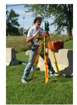
Figure 5. Photo. Reflectorless Total Station
