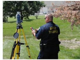
**Figure 6. Photo. Semi-Robotic Total Station** Source: Kansas Highway Patrol and CSI Mapping
