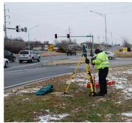
Figure 7. Photo. Robotic Total Station
