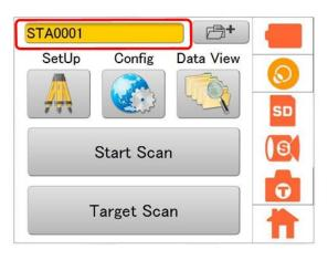
Not only for the first station SetUp, a new station point name should be entered each time the instrument is moved, or a new scan is started at the same station point. Each setup within this procedure is known as a Scan Session.
