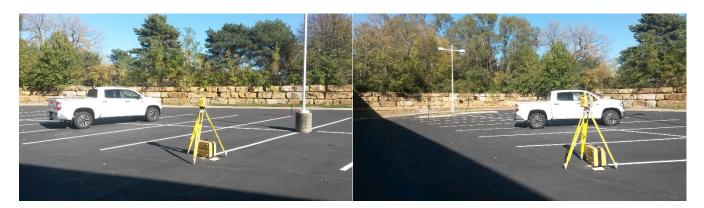
In this particular project, we have opted to set up a target or prism on the next point of our traverse. Turn the GLS-2000 scanner to the next point in your setup, then press the Target Scan button. You will use the  $\Leftrightarrow$  button to switch between tele lens and wide angle lens, and the zoom in/zoom out buttons to zoom in & out on your screen.
