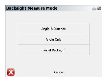
When shooting to your backsight you have two options available and they can be accessed from the <u>instrument toolbar</u> using the Mapping Method button. The measure modes available are described as follows:
