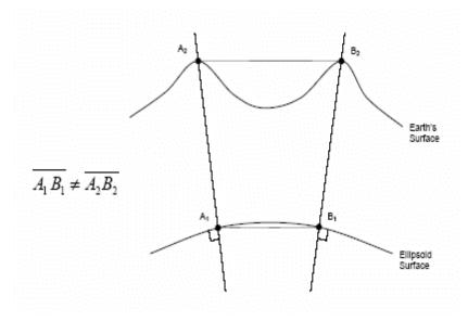
Figure 1. Divergence of Ellipsoid Normals.
