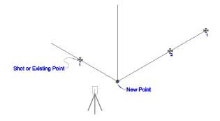
An example of where you could use this is to pick up the corner of a building, whose corner cannot be scene from the total station. You could take two shots on one wall to define the reference line, and then take another shot on the intersecting wall. A perpendicular intersection will be computed, which in this case would be the corner of the building.
