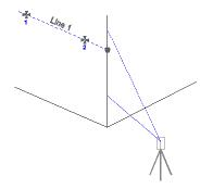
An example of where you might use this is to locate the corner wall of a building. Simply shoot two points on one of the walls, then turn the instrument so it is pointing anywhere along the corner of the building. This command is intended to be used with reflectorless total stations.
