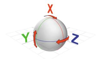
We recommend to perform both calibration procedures on regular basis to ensure the reliability and accuracy of the Electronic Bubble. Magnetic Sensor may require more frequent calibration than tilt sensor depending on your calibration location and distance travelled. Consult with your GNSS receiver manufacture representative for more information regarding calibrate internals.
