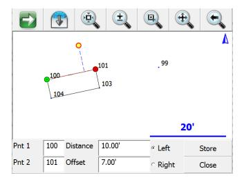
In this example, the baseline is from point 100 to point 101. You will see that an orange dot is displayed in the drawing at the location defined by the point 10m down the baseline and offset 7m to the left.
