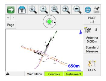
On the GNSS Measurement Screen, if the Tilt Rejection is turned on and current tilt angle exceeds the preset rejection value, the Store Position button will be deactivated and GNSS measurements will not be averaged until the GNSS receiver turns to a plumb and stable position.
