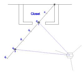
After you take your two measurements, all you need to define is the offset distances. In this example, the corner is two feet to the right of the first measurement (point 1), and 8' up from the floor. After you define the offset directions and offset amounts, you can press the **Store Pnt** button to store the new point.
