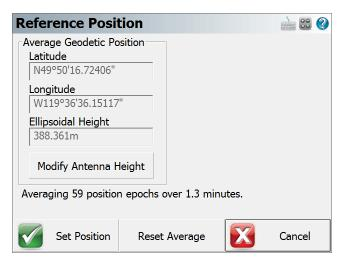
It is up to you to determine how many observations or the duration of time you want to wait before accepting the averaged position. At any time you can restart the process by pressing the **Reset Average** button.
