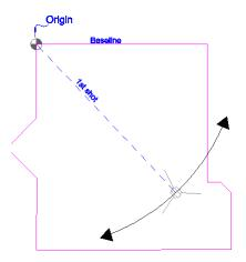
Then using the second shot, the total station location in the room can be accurately computed.
