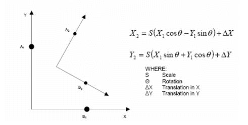
Figure 2. Horizontal Four Parameter Transformation.
