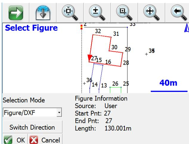
Whichever Selection Mode you use, the selected line will be highlighted in red in the map screen along with a direction indicator. If necessary, you can press the **Switch Direction** button to reverse the start and end of the selected line. Press OK to accept the selected line and proceed to the next step.
