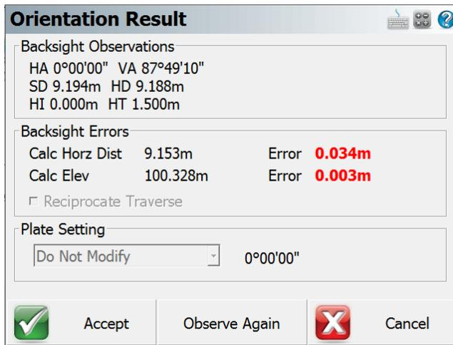
The backsight point that will be stored will be based on which point you selected in the Information screen shown above, which by default is the first reference point you observed. You do not need to take another measurement to the backsight as it has the original measurement you made. At this point you can do the following:
