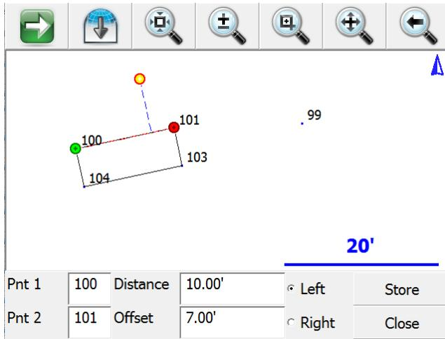
In this example, the baseline is from point 100 to point 101. You will see that an orange dot is displayed in the drawing at the location defined by the point 10m down the baseline and offset 7m to the left.
