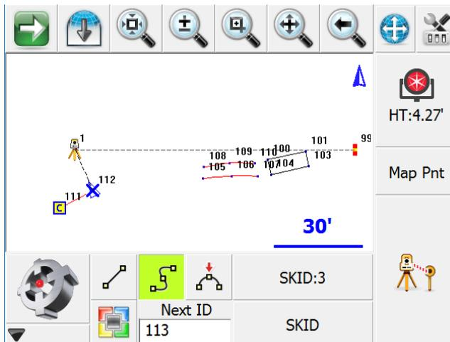
Note the insertion of ":3", this is the group number. Re-use of the Description SKID for a new line series in the current Scene will automatically increment the group number by one. This allows you track and store multiple active lines of the same description without the need for multiple entries in your AutoMap Library. For example, SKID:2, SKID:3 ... SKID:n can now be replaced with a single SKID entry.
