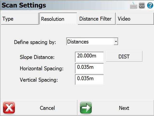
The image shows the 'Scan Settings' dialog box with the 'Resolution' tab selected. The 'Define spacing by:' dropdown menu is set to 'Distances'. Below this, there are three input fields for spacing values and a 'DIST' button:
