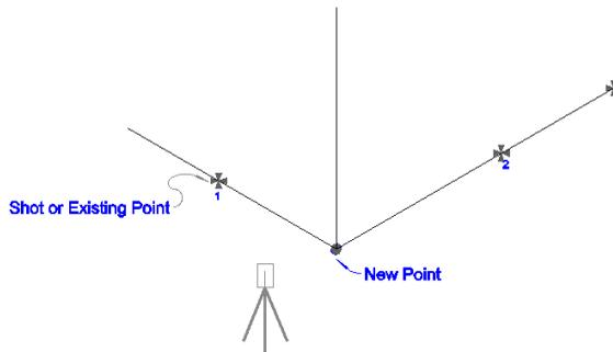
An example of where you could use this is to pick up the corner of a building, whose corner cannot be seen from the total station. You could take two shots on one wall to define the reference line, and then take another shot on the intersecting wall. A perpendicular intersection will be computed, which in this case would be the corner of the building.
