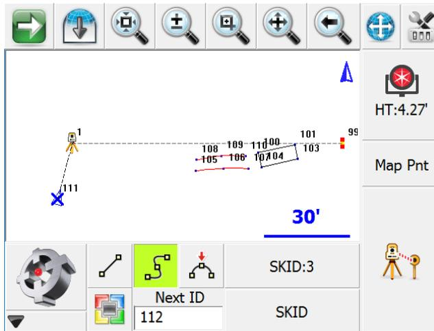
After the second point for this line has been recorded, the first segment will be created. From this point forward, simply continue taking shots to add to the now current Active Line: SKID:3
