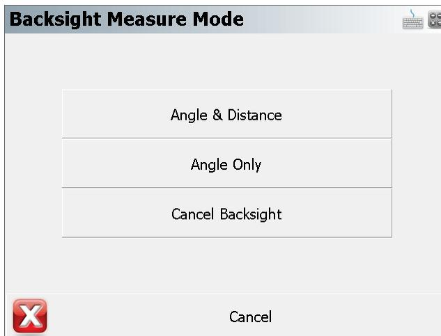
When shooting to your backsight you have two options available and they can be accessed from the [instrument toolbar](#) using the Mapping Method button. The measure modes available are described as follows:
