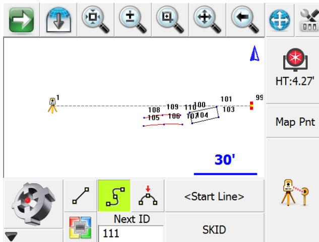
After the measurement to the first point for the new line is complete, the line will be added to the Active Lines list, identified by the current point description and an automatically assigned group number: SKID:3. The group number is three, because this is the third figure using the description SKID.
