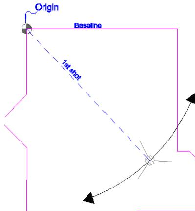
Then using the second shot, the total station location in the room can be accurately computed.
