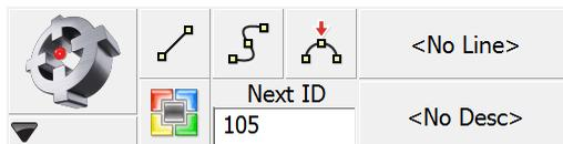
The Topo Toolbar is used to help automate linework as well as show you the description and next point number for your shot. Just like previous versions of Evidence Recorder you can control your linework by tuning on and off the line, arc and curvy toggles. There is also a user-programmable button that can be customized to start any command.
