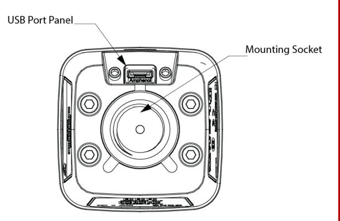
Figure 3: Micro-AB USB Port Panel
