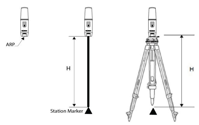
Figure 24: Obtaining Accurate Antenna Height
