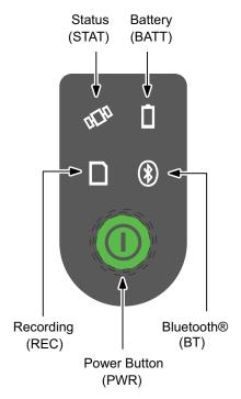
Figure 4: LED Display Panel
