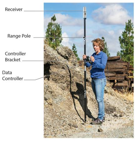
Figure 23: RTK Rover
