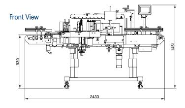
The dimensions shown are for standard machine. The conveyor can be extended: the length may vary based on selected options. This machine can run independently or be integrated into an automated packaging line. All CVC equipment is covered by a one-year parts warranty. Full Warranty details are included in our equipment proposals or can be found on our website.
